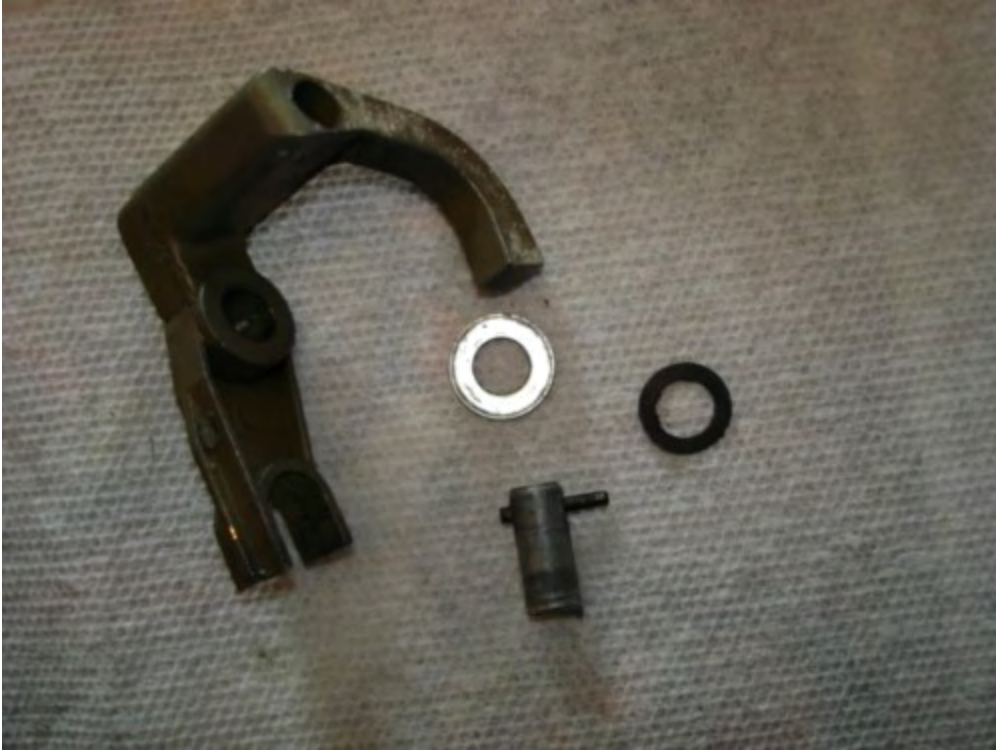
So here's the L shaped striker, the two washers and what's left of the metal pivot.
